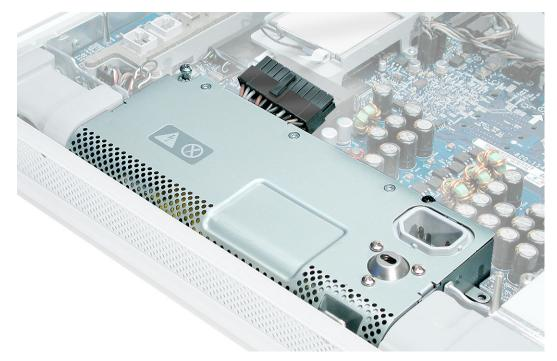
4. Connect the black power supply connector and tighten the two captive screws (the middle screw and the screw on the left), turning them clockwise. Replace the remaining screw on the right.
