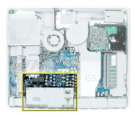
3. Remove the screw on the right and loosen the other two screws by turning them counterclockwise five to eight revolutions. **Note:** The middle screw and the screw on the left are captive; they will not come out of the power supply.
