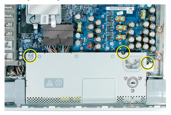
5. Turn the middle case screw counterclockwise about five revolutions. This step prepares the back cover to be installed and secured.
