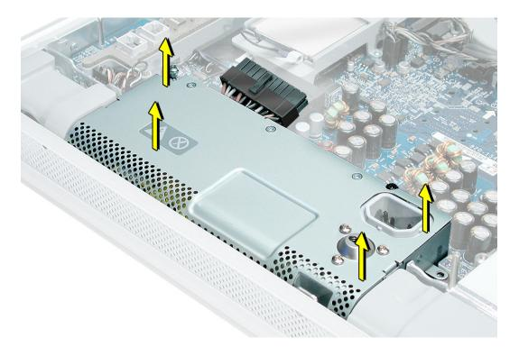
8. Tilt up the power supply until it clears the edge of the main circuit board. Lift it out of the computer and set it aside.
