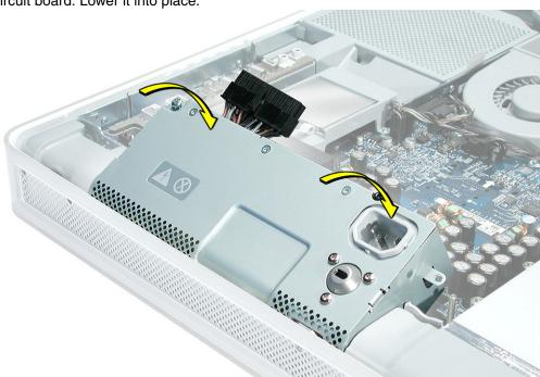
3. When the power supply is installed properly it should be flush with the gray plastic parts on the right and left sides.
