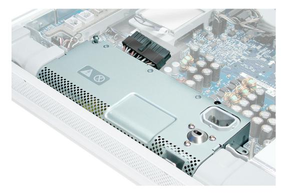
6. To unlatch the power supply, tighten the middle case screw by turning it clockwise five to eight revolutions.
